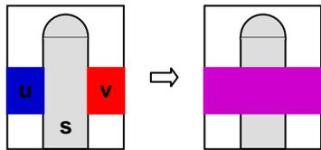
(d)  $\{=, =\}$ : Slots u and v have two pairs of coplanar side faces.
