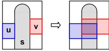
(b)  $\{<, <\}$ : Slots u and v have no pairs of coplanar side faces.
