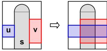
(a)  $\{<, >\}$ : Slots u and v have no pairs of coplanar side faces.
