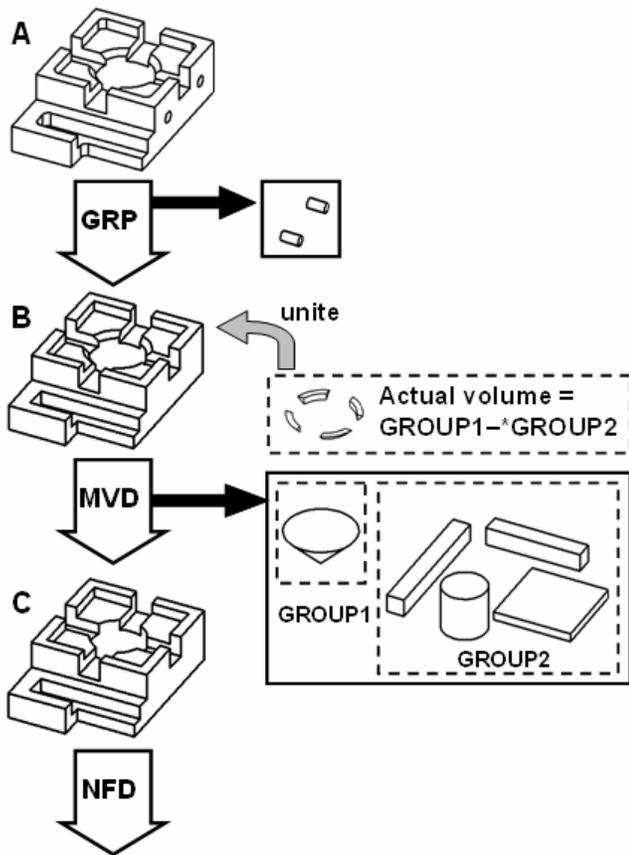
Figure 2. Hybrid feature recognition for Part A
