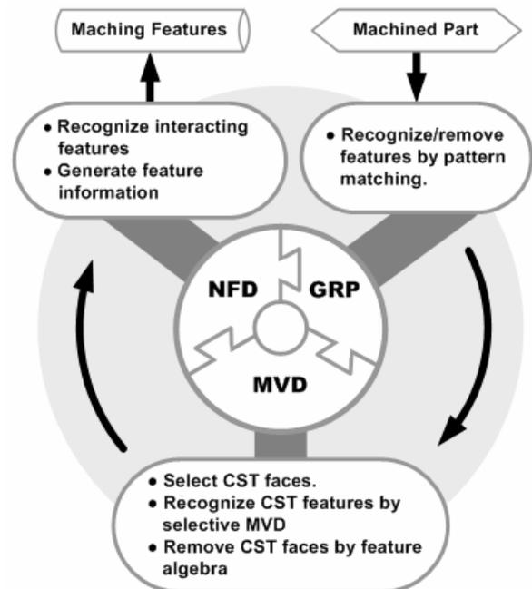
Figure 1. Hybrid feature recognition system
