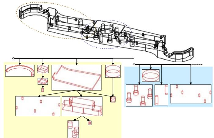
Figure 8. Recognized features for change arm part
