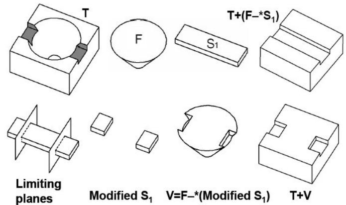
**Figure 5. Curing anomaly type 1**
