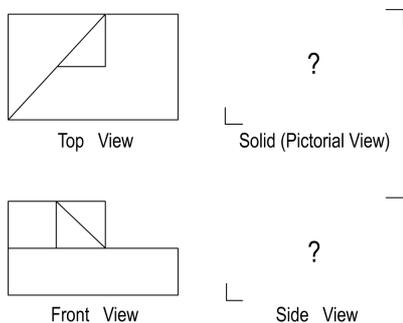
Figure 2: Example of a Missing View Problem
